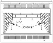
Figure 13 - Removing Firebox Bottom
